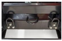
**Lifiting points and towing hook** Once the skip is in the raised position, you can use the 4 lifting hooks to lift the machine. A towing hook is also avalaible at the back of the chassis.
