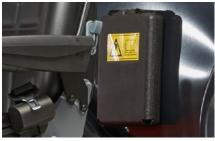
**Compartment for documentation** Waterproof and lockable compartment is also avalaible on the machine. You can use it for instance with user and technical manuals.
